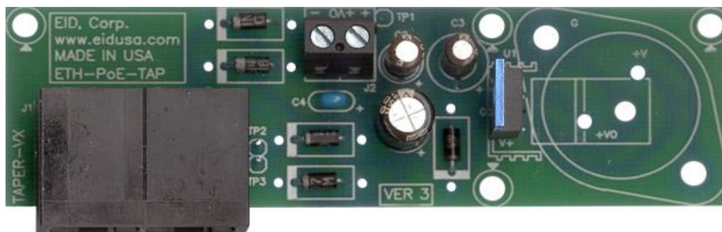
TAP PS for remote location with power regulator
