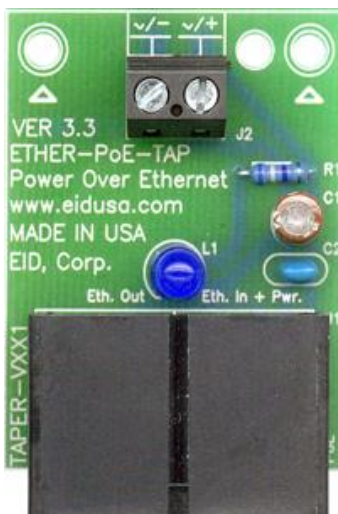
TAP PS for remote location with power regulator
